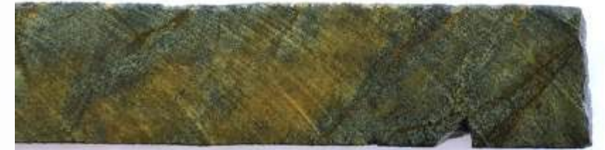
ADD007: 92.00 m-93.00 m core sample interval with 33.40 g/t Au
