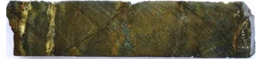
ADD004: 58.00 m-59.00 m core sample interval with 20.90 g/t Au
