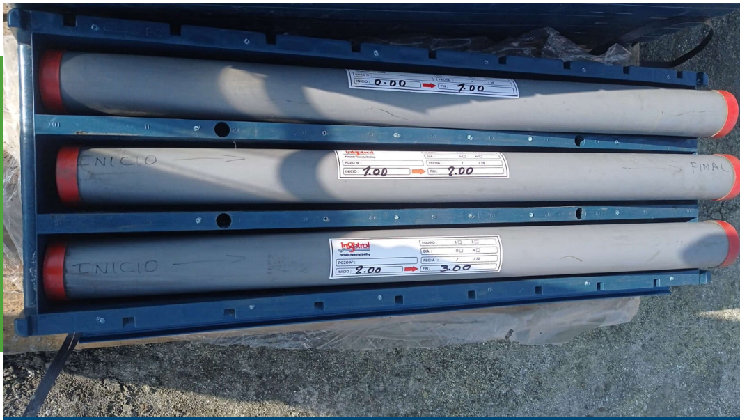
First drill samples from Quilacocha Tailings ready for shipment to Bureau Veritas
