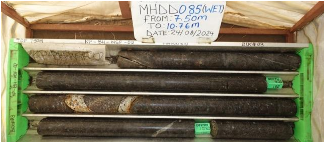
Shallow fresh bedrock at the Water Storage Facility dam wall location
