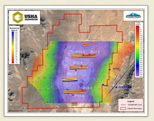
Project target is a strong conductive geophysical anomaly identified through gravity and controlled source audio magnetotellurics/ magnetotellurics (CSAMT/MT) surveys
